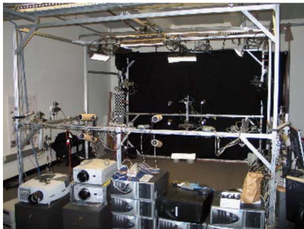
(a) Multi-camera stereo system
