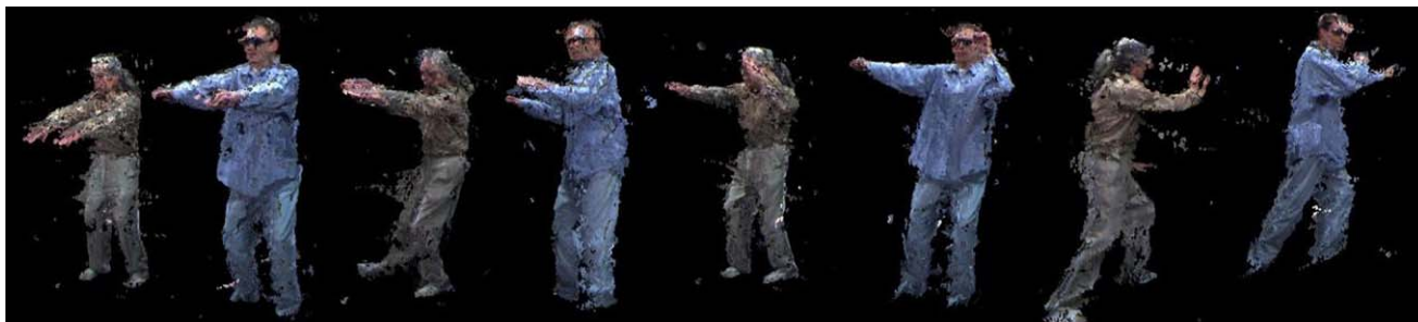
Fig. 1 A student (right, in blue shirt) is learning the tai-chi movements by following pre-recorded 3D TI data from a tai-chi teacher. These images (both the student and the tai-chi teacher) are rendered from the reconstructed 3D points using our tele-immersion system
